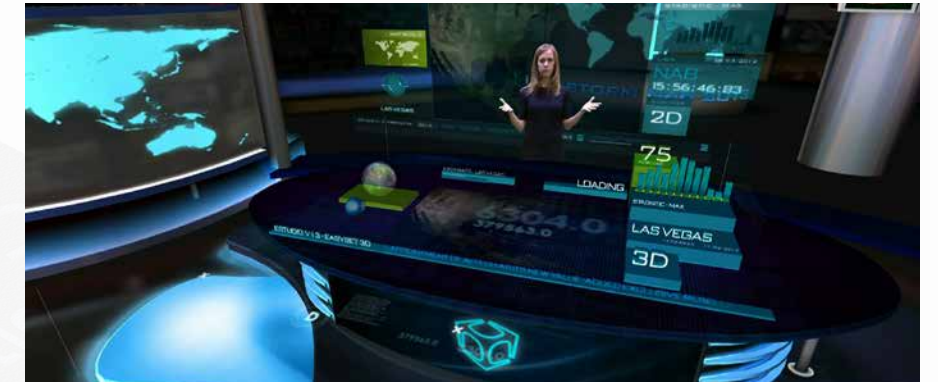
In Trackless virtual sets the talent is just a flat sticker with limited movements
